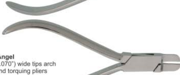
DE-1339 Tweed / Angel 1.78mm (.070") wide tips arch forming and torquing pliers
